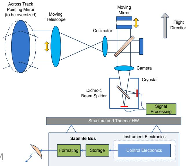
Instrument functional block diagram
