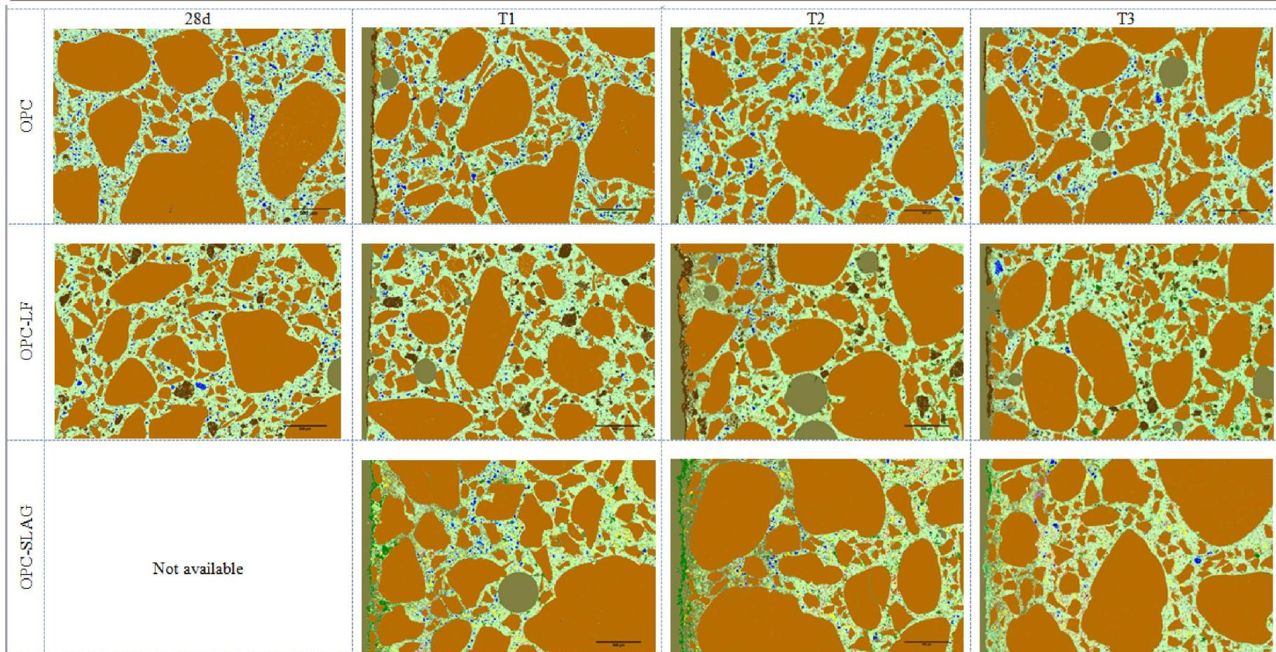
Figure 5: Classified images of OPC, OPC-LF (Limstone Filler) and OPC-Slag at 28, 250, 350 and 720 days, corresponding to previous BSE images (Figure 3).
