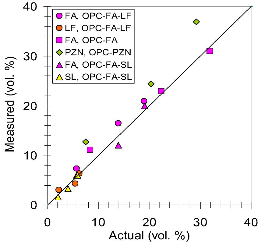
Method shows excellent results on fly-ash, limestone, slag. Discrepancy on pozzolan due to clay impurities.
