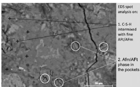
Fig. 2. Example of EDS spot analysis on C-S-H and Afm/Aft phases in the pocket for PC samples.
