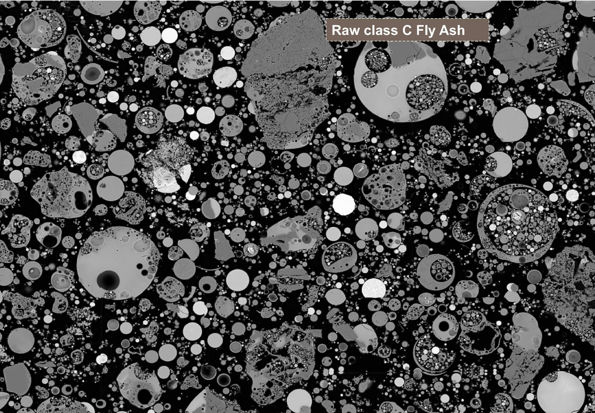
A high-magnification micrograph showing a dense population of fly ash particles. The particles vary in size and shape, ranging from small, uniform spheres to larger, irregular, and porous structures. Some particles exhibit internal porosity or contain smaller voids. The overall texture is granular and somewhat chaotic.
