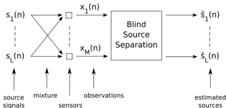
Figure : Blind source separation problem ( $L$  sources and  $M$  observations ( $M \geq L$ )).
