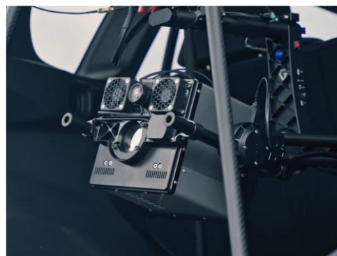
Fig 2. Close-up on the Hyper-Cam Nano optical head.
